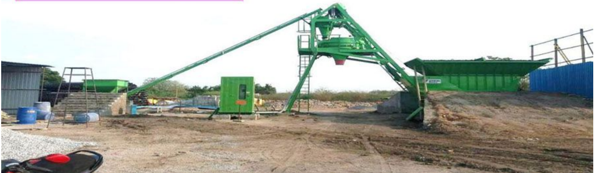
Batching Plat – 30 Cum Capacity
